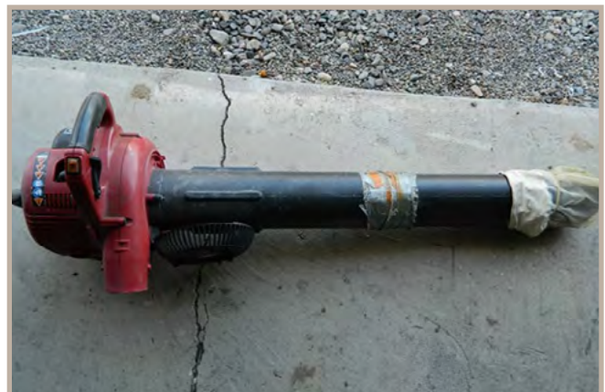
Figure 6. An inverted leaf blower or DVAC for collecting insects. The open end is covered with a mesh secured with a rubber band. It works as a vacuum by sucking up and trapping insects in the mesh.
