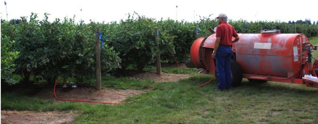
Fig. 10. Modified orchard air-blast sprayer injection.
